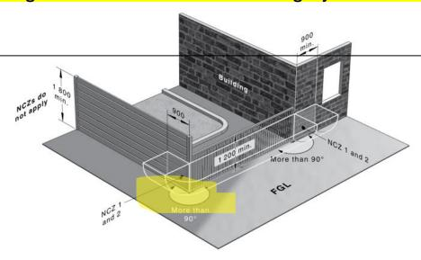
Figure 2.3 — Intersecting internal barriers
