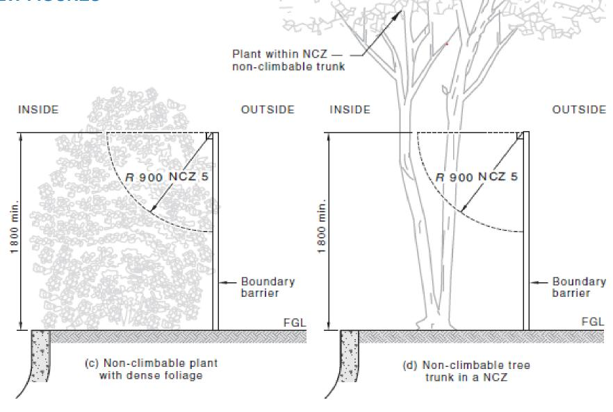
Figure 2.6 — Example of non-climbable plants within NCZs — Boundary barrier
