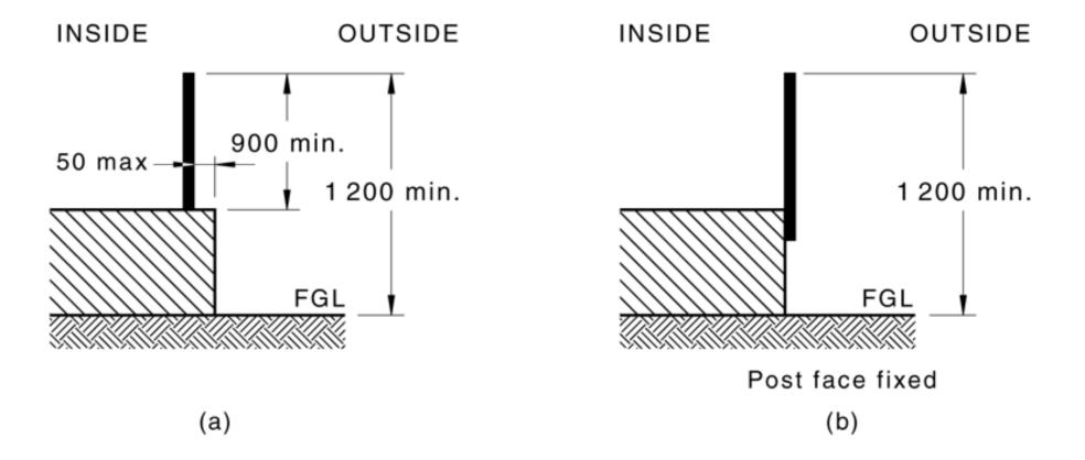
Figure 2.17 Fixing for a composite barrier
