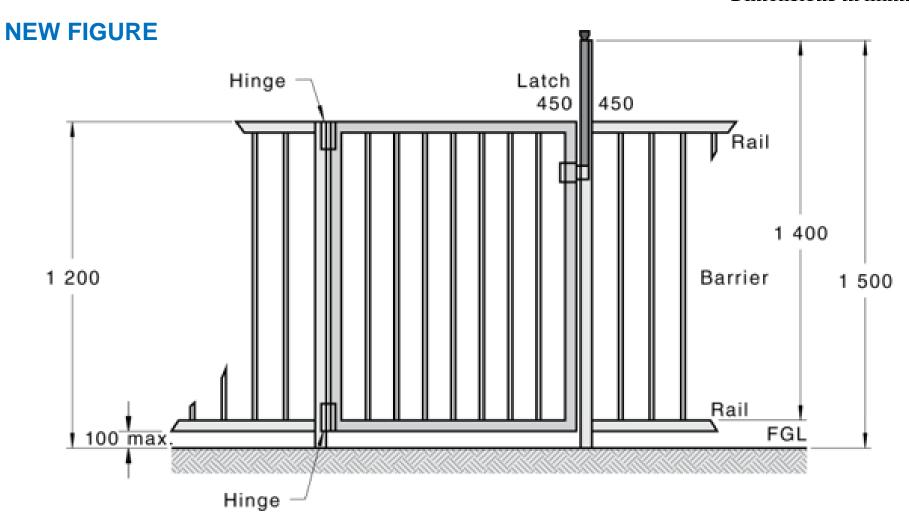
Figure 2.19 Example of latch release 1 500 mm or more above FGL
