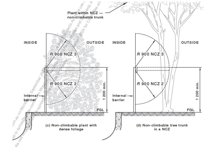
Figure 2.5 — Example of non-climbable plants within NCZs — Internal barrier
