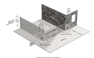
FIGURE 2.3 INTERSECTING INTERNAL BARRIERS
