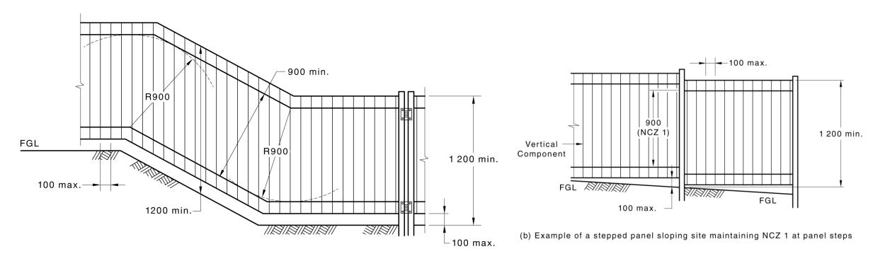
(a) Example of a 900 mm radius maintaining NCZ 1 along the length of a barrier on a slope
