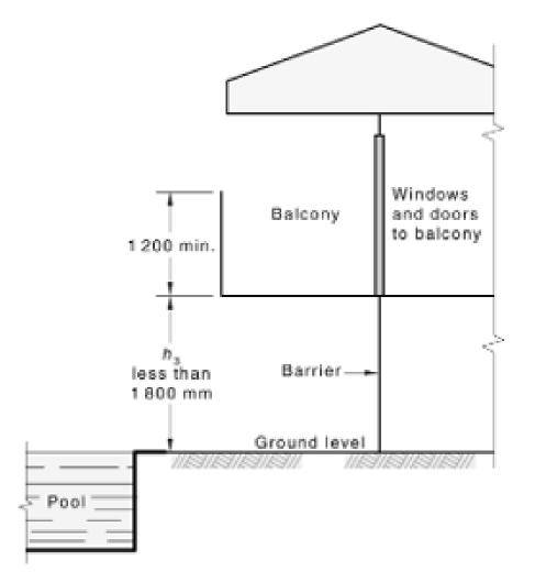
Figure 2.25(A) — Balustrade used as a barrier
