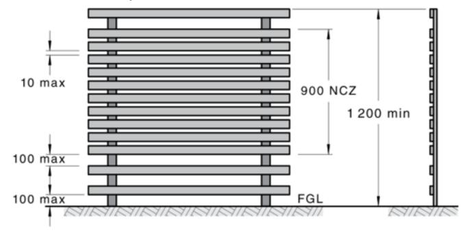
Figure 2.12 Example of horizontal slat construction for barriers of minimum height 1 200 mm
