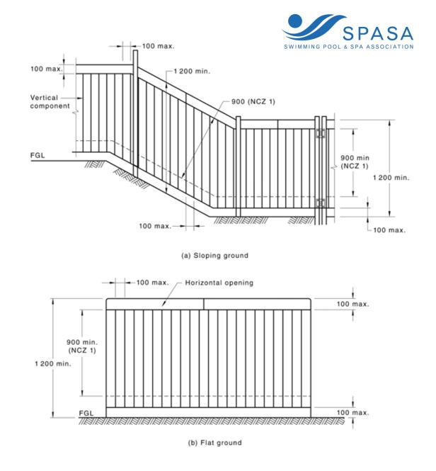
Figure 2.13 Examples of openings in a barrier
