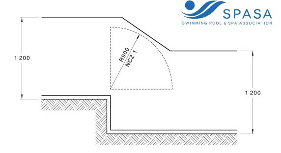
(b) Example of maintaining NCZ 1 on a raked glass barrier over stepped ground
